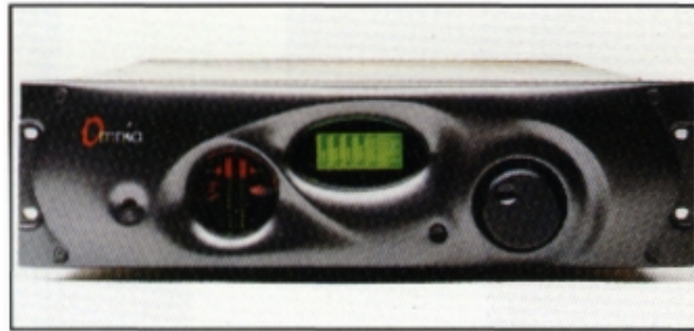
AT A TOUCH: Control of the Omnia.FM is through a large front panel dial.
