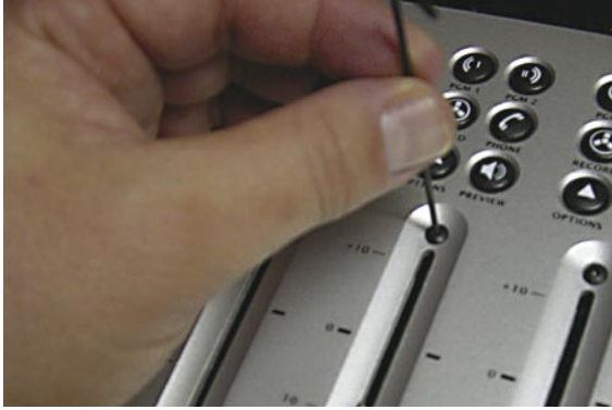
Figure C-7: Loosening hex screws
