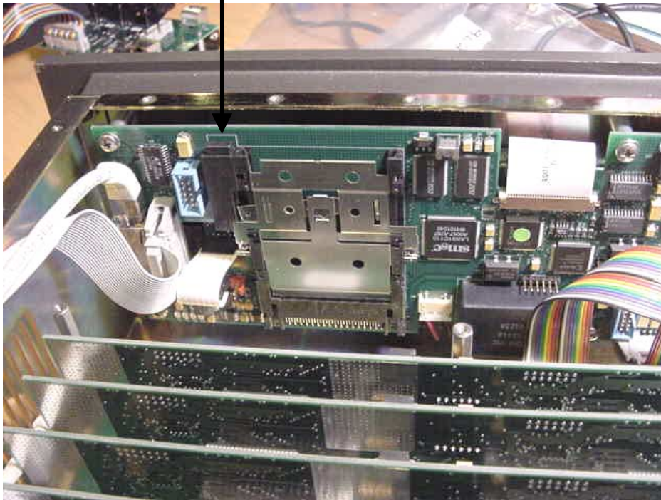
Rear view of the front-panel controller card with the Omnia 4.5's top cover removed. The PCMCIA memory card slot is shown empty.
