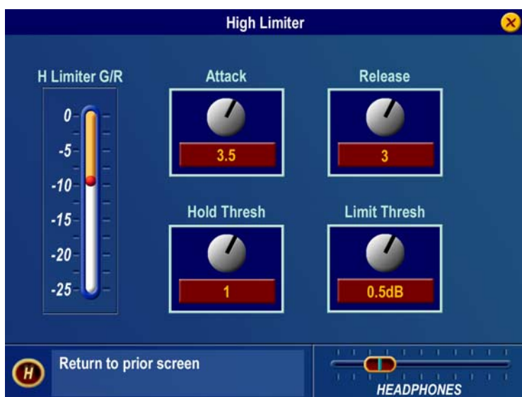
Limiter Submenu – High Limiter shown as example (the Limiting G/R meter is displayed in the page along with the controls)
